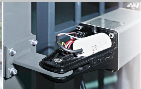
Capacitor fixed into place
